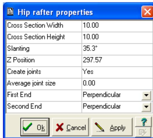
Enter the purlin width, angle of incline, end cuts and joint size in the dialogue. Joints can be turned off to speed up generation, as this reduces the amount of computation required.
