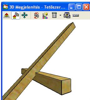
A step joint can be used for example when joining rafters and purlins. When joining two elements you may also an incision value in the dialogue.
